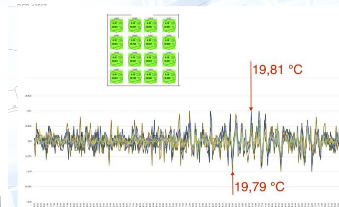
Measurement recorded of the temperature stability: room temperature with filter fan units
